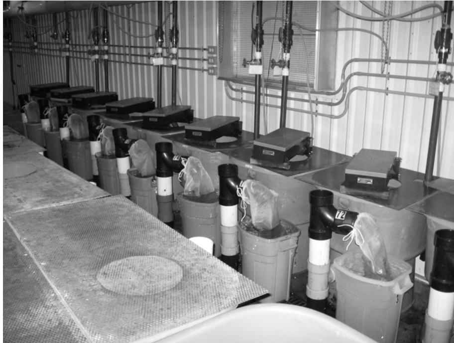
Figure 1. Tank display showing the feces collectors and automatic feeders
